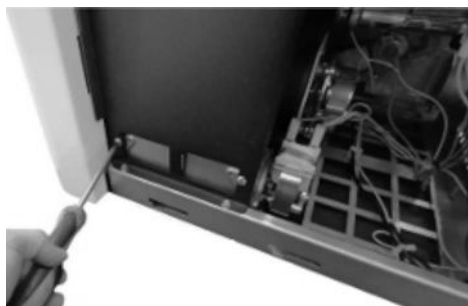
Fig. 78 - Reiniging omgevingsventilator (Atena³ Plus 12/14 - Duke 12/14 At - Saba 12/14)
